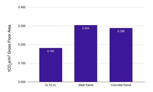
The comparison materials (steel frame and concrete frame) were selected in order to reflect how the building would have realistically been built as a more typical approach of today's architecture. The material's embodied emissions (graph above) take into account the Cradle to Gate Life Cycle Assessment per m<sup>2</sup> of the gross internal floor area (22,890 m<sup>2</sup>).
