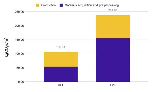
The above graph illustrates the results of the cradle to gate LCAs of CLT and LVL (excluding biogenic emissions). The results show that CLT has the lower impact per m<sup>3</sup> at 107 kgCO<sub>2</sub>e/m<sup>3</sup>, while LVL is higher in both the material acquisition and preprocessing and the production stages (totalling 238 kgCO<sub>2</sub>e/m<sup>3</sup>).
