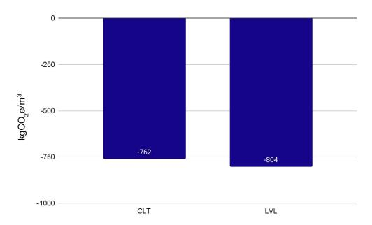
Biogenic emissions are -762 kgCO<sub>2</sub>e in the CLT and -804 kgCO<sub>2</sub>e in the LVL. There are different factors that would be affecting these results, for example, the LVL has a lower percentage of moisture content but a higher density of woody biomass at that percentage.
