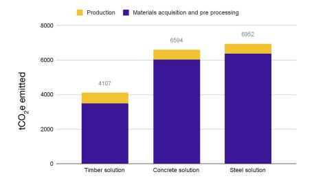
The results show that based on the emissions from the cradle to gate of the material, **the timber solution (CLT/LVL) is by far the lowest carbon solution.** If the biogenic carbon stored in the wood harvested for the product was considered, it would result in a negative value of  $-895.3 \text{ tCO}_2$  e for the materials acquisition and preprocessing and production stages.
