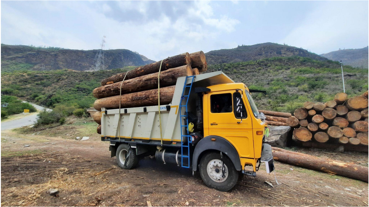
Figure 9 Timber transportation by Trucks (10 m 3 Capacity)
