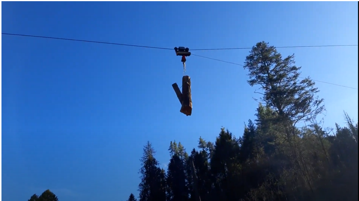
Figure 6 Skyline Cable Cranes at Dawathang FMU, Bumthang
